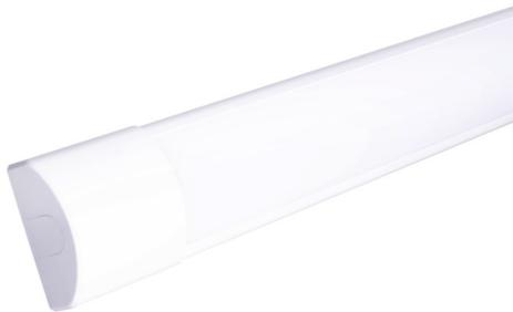
The Nova III Tri Colour slim batten is a Class I product and must be earthed. Colour temperature is switchable between 3000K, 4000K & 6000K at the time of installation by operating the switch at the opposite end to the mains input of the Nova III Tri Colour. Featuring loop in and out. CE Approved. 220-240VAC. 50/60Hz supply. IP20 rated. Temperature rating: 10°C to 40°C. Available in 4ft, 5ft & 6ft. 40 Watt, 50 Watt & 60 Watt Epistar LED's.
