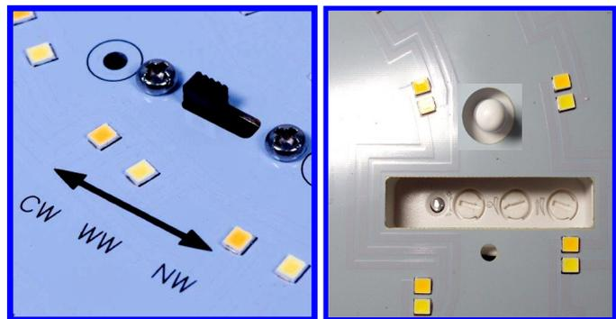
**Settings** There are 3 settings that can be adjusted by turning the dials on the sensor.
